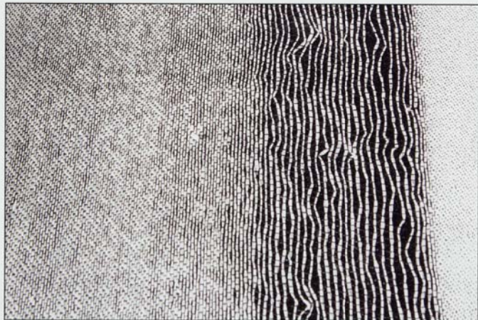
Above: Thalassa fabric inspired by images of the sea and waves. Thalassa means sea in Greek. Fabric prototype for interior textiles. Woven on a computerized jacquard loom using cotton and paper yarns. The variations on the weft density were achieved by manually changing the weft ratio whilst weaving. Ismini Samanidou
